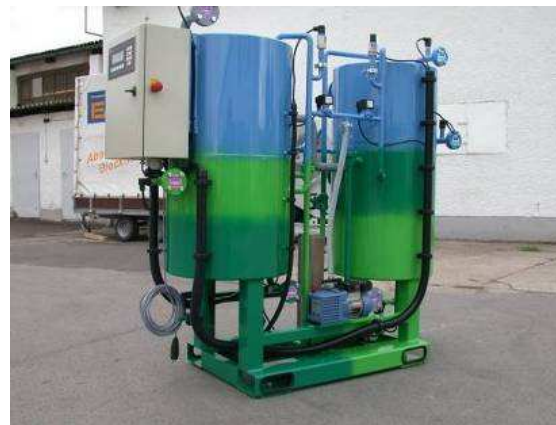
Figure 1 - EAW 15 kW absorption chiller
